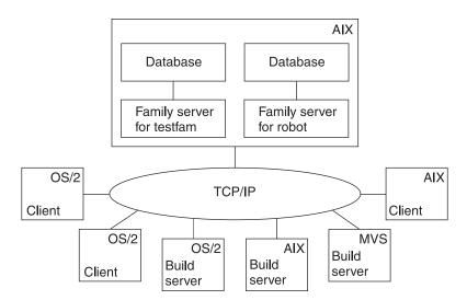
Figure 1. A sample TeamConnection client/server network
